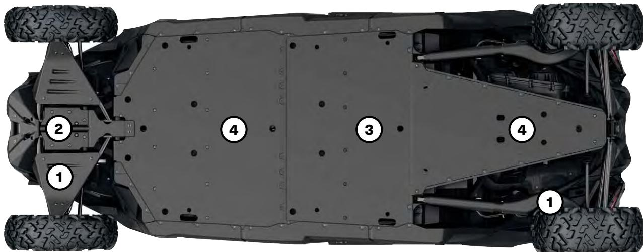
**Our plastic plates glide smoothly and silently over obstacles, offering great protection in rough terrain. Made of abrasion-resistant thermoformed  $\frac{3}{8}$ " (10 mm) thick High Molecular Weight Polyethylene (HMWPE).**
